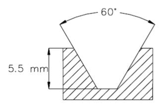
**9.2.2** The sum of the width of the grooves encountered by a circumferential line in the area described above must be at least 4 mm.
